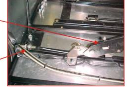
By adjusting the nuts on the handbrake (as indicated), the tension to the handbrake can be adjusted accordingly. It is recommended that the tension be set so that the handbrake begins to take after 2 'clicks' and that it is fully engaged after 4 to 5 'clicks'.
