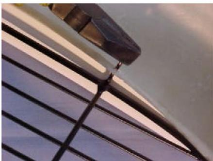
2. Using a non-abrasive, non-corrosive contact adhesive, apply the bonnet rubber to the nose cone in its original position (Refer to step 6 of the above procedure.)
