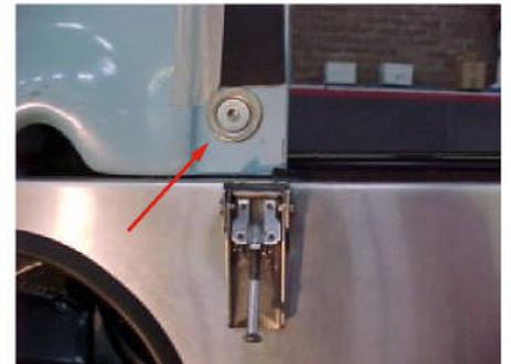
3. Tilt the nose cone up and away from the chassis.
